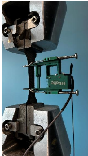
Figure 1 - Universal testing machine with a material sample clamped in place and an extensometer attached
