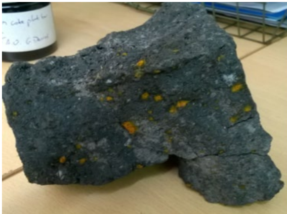
Figure 25 - Iron contamination in coke sample (note orange spots) (Waters, 2018)
