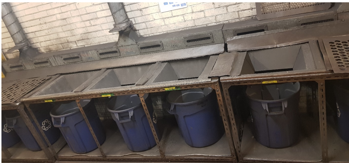
Figure 37 - The micum screening bench with screens removed used for mixing coke samples (Waters, 2018)
