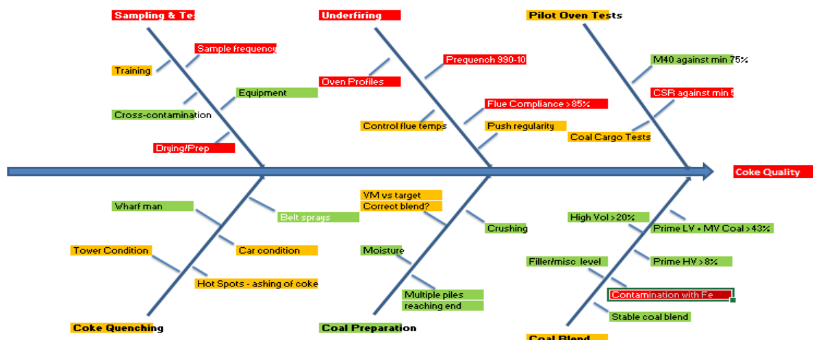
Figure 24 - Root cause analysis of coke quality variation carried out at coke ovens (Dickinson, 2018)
