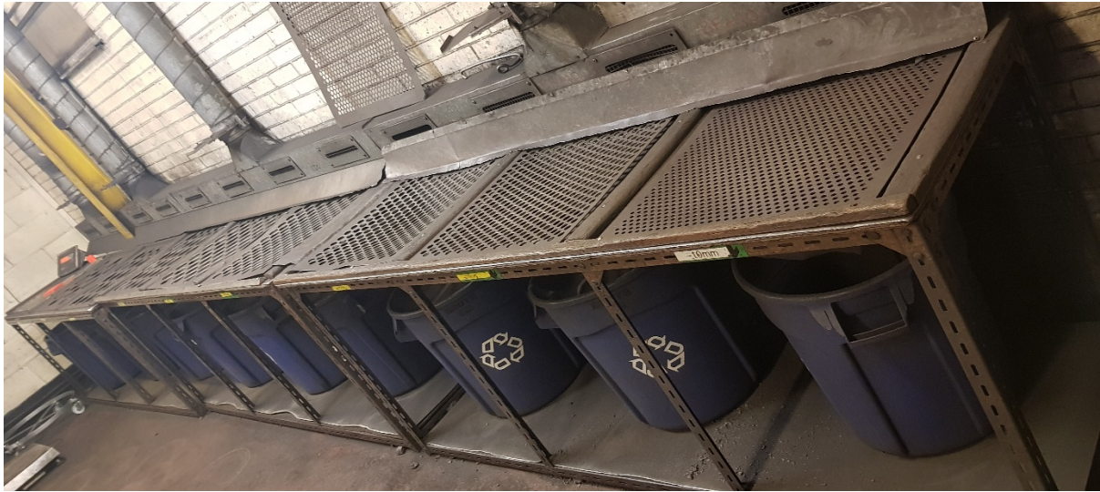
Figure 7 – Coke particle sizing screens (Waters, 2018)
