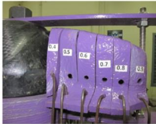
Figure 25 - Segmented loading test supporting structures (Kumar et al., 2019)
