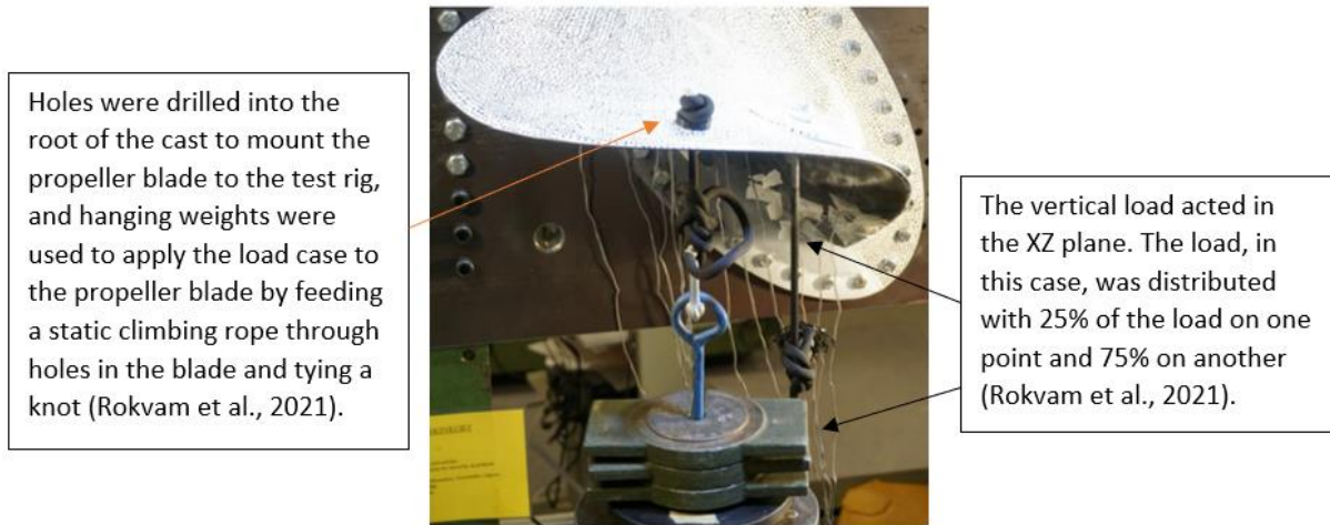
Figure 20 - Image showing loading of the blade (Rokvam et al., 2021)
