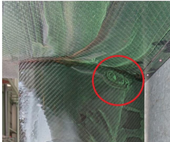
Figure 29 - Wing Lower Surface Flow Visualisation Paint Test
