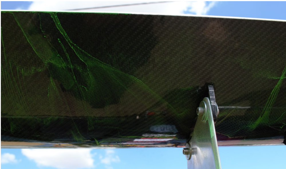
Figure 34 - MCR Sports 2000 Rear Wing Mount Interaction Flow Visualisation
