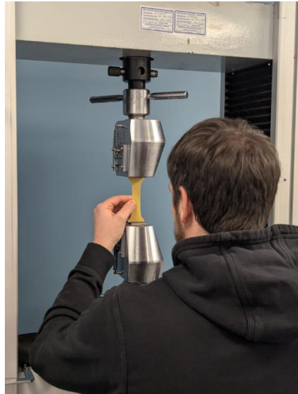
Figure 2 – Setting up of test sample in Denison machine
