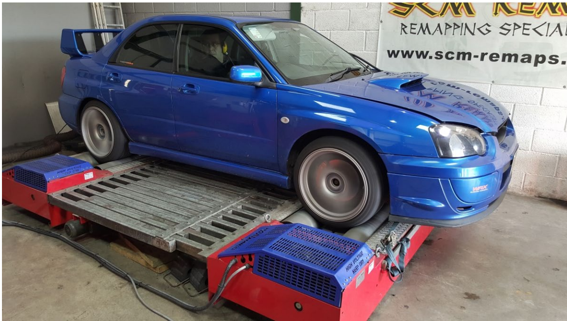
Figure 12 Dyno featuring double roller (SCM Remaps, 2019)
