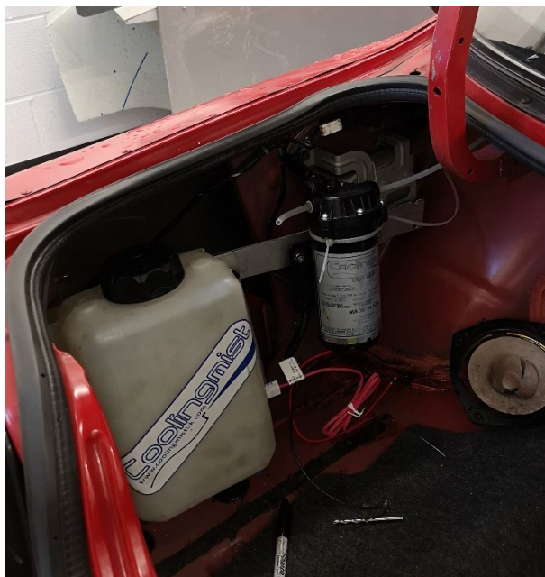
Figure 22 Photograph showing Water/Methanol Installation in vehicle
