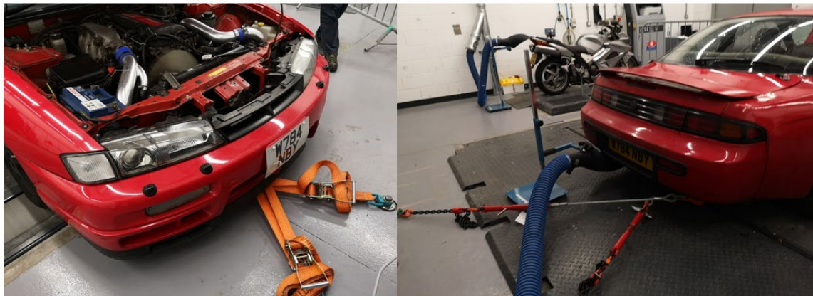
Figure 16 Photograph of S14 securing points on dyno
