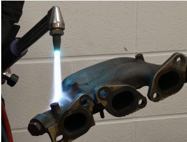
Figure 18 Photo of exhaust manifold being welded
