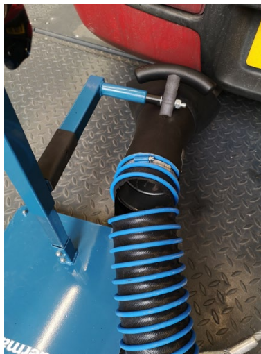
Figure 17 Photograph showing failed exhaust extraction hose
