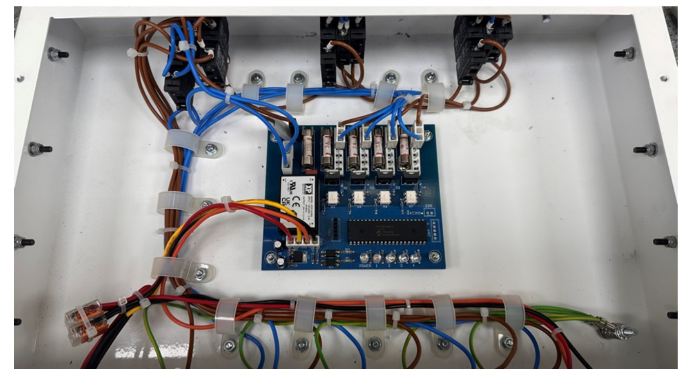
Figure 4 - Enclosure wiring with the PCB, switches and external connectors
