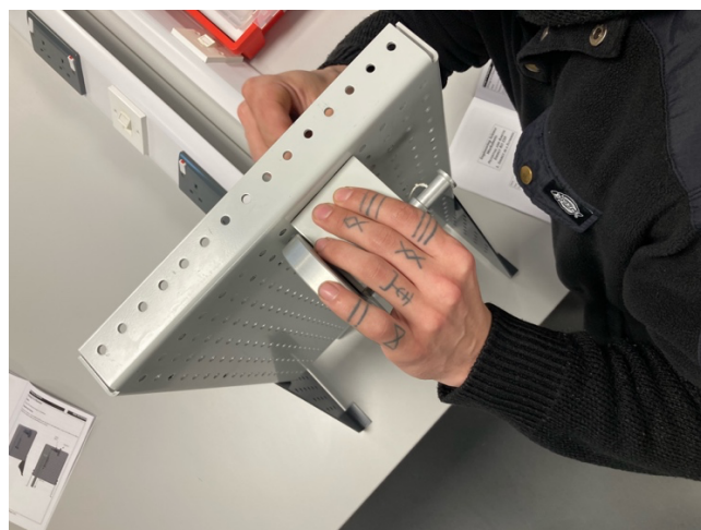
Figure 2 Mounting of bearing block to steel plate
