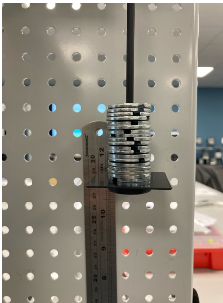
Figure 4 Positioning of weight hanger at 280mm above rest position
