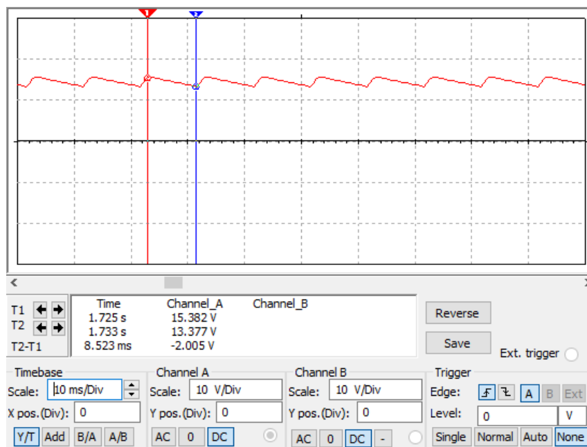
Figure 18 - Full-Wave Bridge Rectifier with Smoothing Capacitor Waveform
