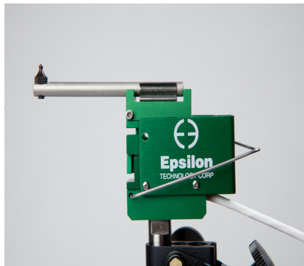
FIGURE 4 - EPSILON DEFLECTOMETER MODEL 3540
