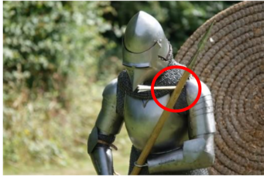
Figure 13 - Experiment Footage Showing an Arrow Penetrating Chainmail with Target Positioned Face on to Archer with Head Down
