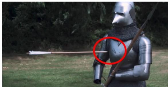
Figure 16 - Experiment Footage Showing Perforation of Plate Armour with The Target Positioned at a Three-Quarter Profile to The Archer
