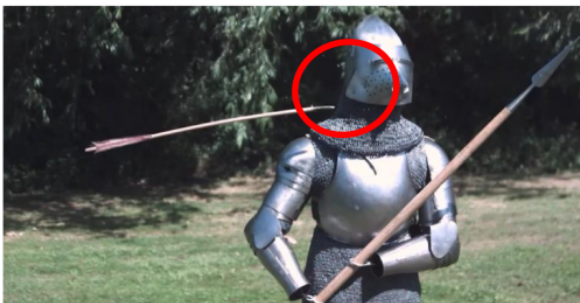
Figure 15 - Experiment Footage Showing a Hardened Tipped Arrowhead Impacting a Helmet with The Target Positioned at a Three-Quarter Profile to The Archer
