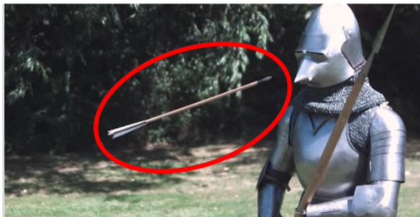
Figure 12 - Experiment Footage Showing Deflection off Padded Chain Mail with Target Positioned at a Three-Quarter Profile to Archer
