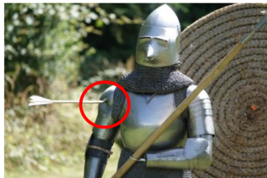
Figure 14 - Experiment Footage Showing Arrow Penetrating Through a Gap in Plate Armour with Target Positioned in a Three-Quarter Profile to Archer
