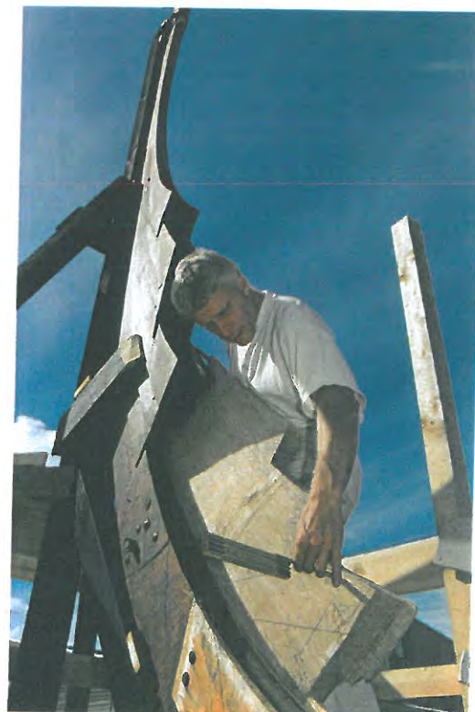
Fig. 1.40 (right). Building the longship reconstruction: the assembly of the keel, stem and hood-ends for the planking. Photo: W. Karrasch.
