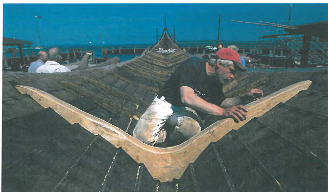
Fig. 1.42. The floor timbers were individually cut to fit the plank shell before being mounted in the ship with treenails through the plank. Photo: W. Karrasch.
