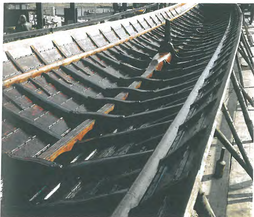
Fig. 1.43. Bottom section of the longship reconstruction amidships, before mounting the beams over the floor timbers and the keelson with its supporting knees. Photo: W. Karrasch.
