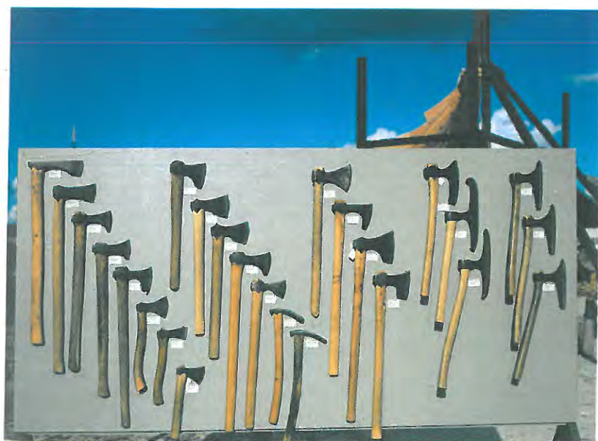
Fig. 1.44. Copies of Viking-Age tools, made for use in the construction process as well as for tool-mark analysis. Photo: W. Karrasch.
