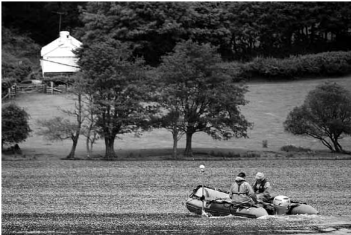
Figure 7.2 Photo of boat on the lake. First echo-sounding survey of Loweswater, 2007. Part of the echo-sounding system is visible over the port side of the boat
