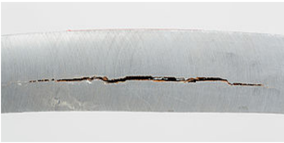
Figure 3: Picture of hydrogen induced cracks
