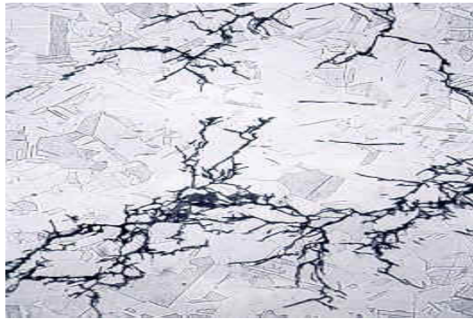
Figure 1: SCC in 316 stainless steel chemical processing piping system (The photo obtained from Metallurgical Technologies)
