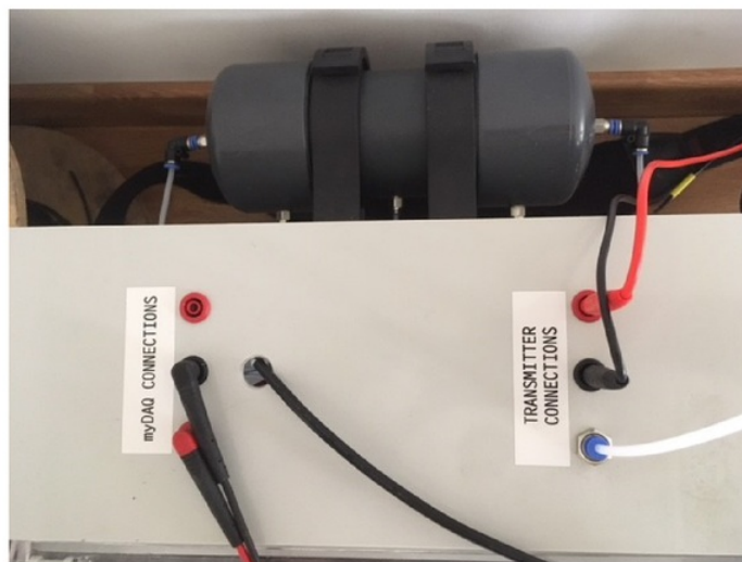
Figure 48 - External Connections & Tank
