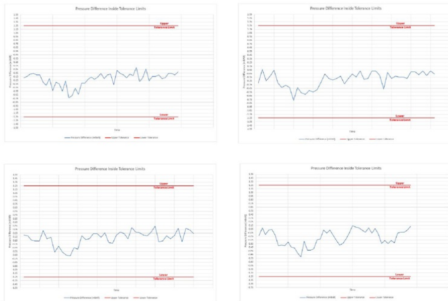
Figure 51 - 4 Tests of Pressure Difference against Tolerance Limits
