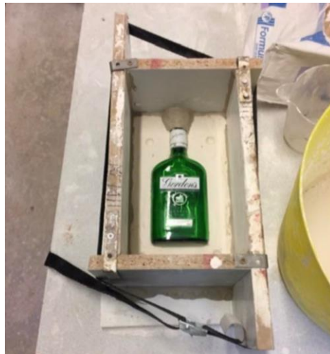
Figure 4: The clay bed is removed and retaining walls are put in place
