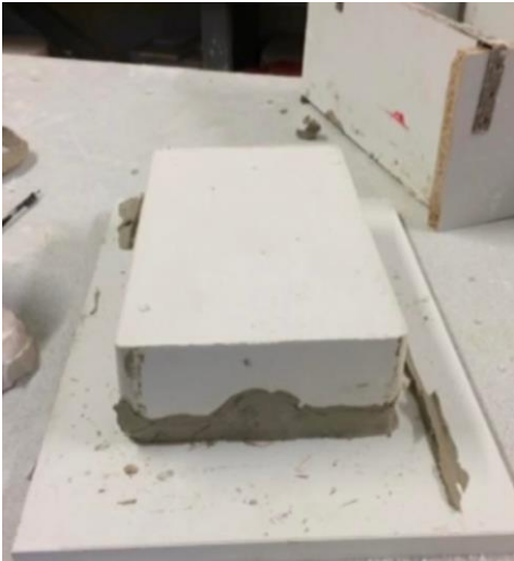
Figure 3: The walls of the mould have been removed, showing the completed mould piece and the clay bed
