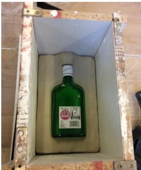
Figure 1: Clay bed is formed around the bottle, and the retaining walls are put in place
