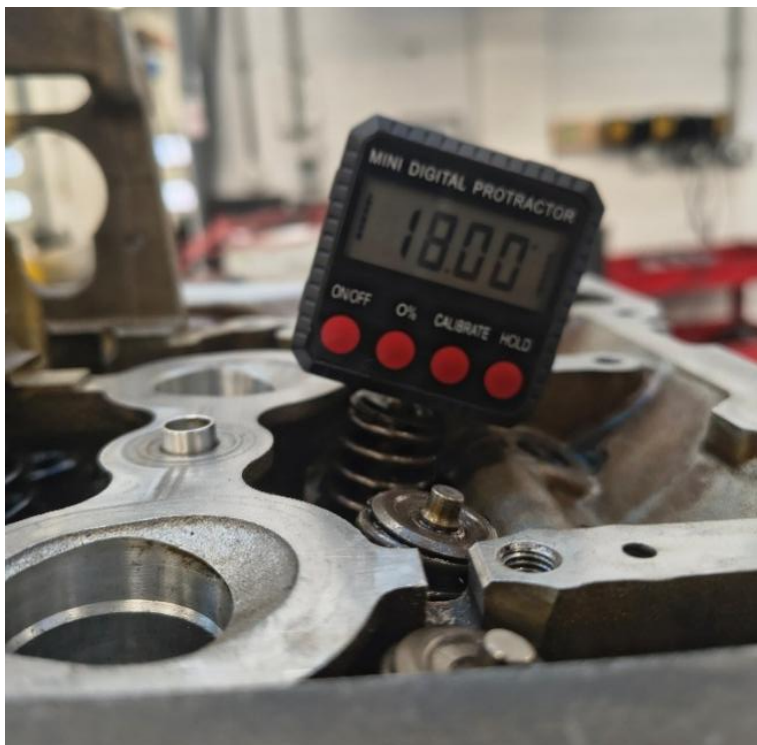
Figure 22: Measuring valve angle
