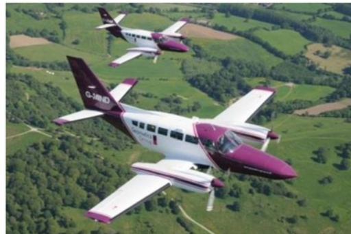
Cessna 404 (G-MIND) & 406 (G-LEAF) Capturing LiDAR Data
