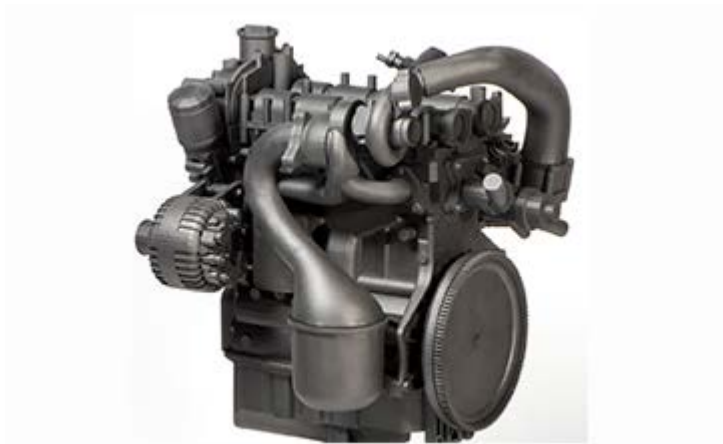
Full size engine 3d printed by graphite
