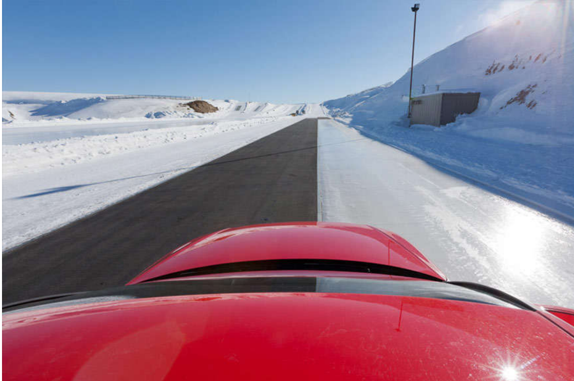
Figure 1: Split mu track (Vehicle Dynamics, 2020)
