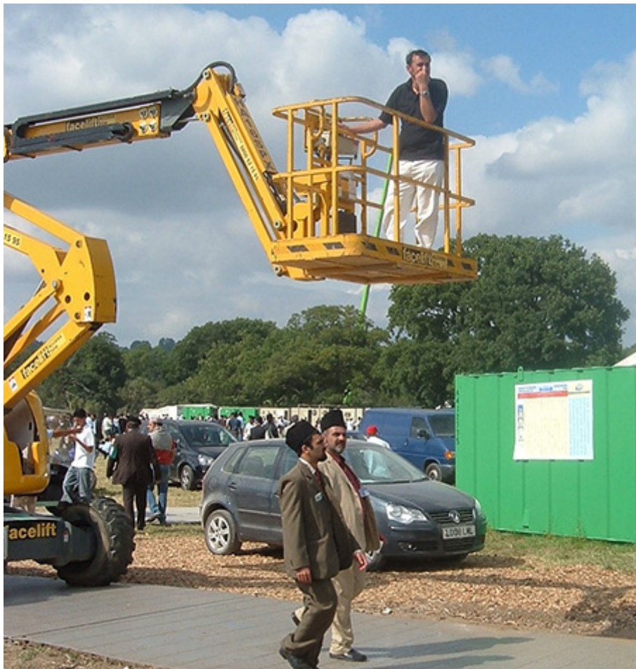
Picture 2: Poor use of a MEWP in the same public area and few minutes later – no risk assessment and training for the user operator
