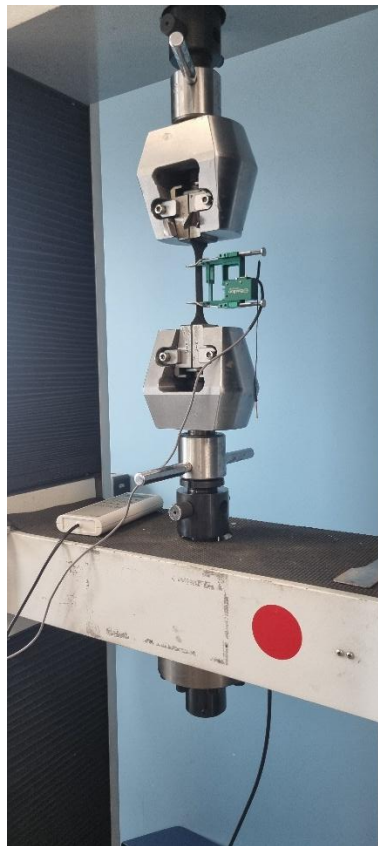
Figure 2: Extensometer connected to gauge section dog bone specimen in during tensile testing.
