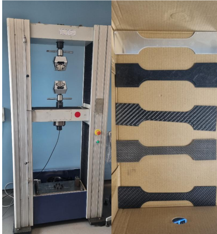
Figure 1: Denison tensile testing machine and dog-bone specimens used for material testing.
