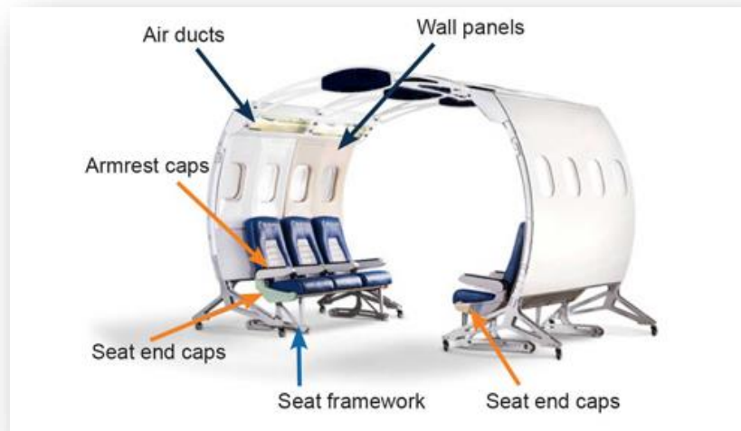
Fig 4 : 3D printing transforming aircraft interior
