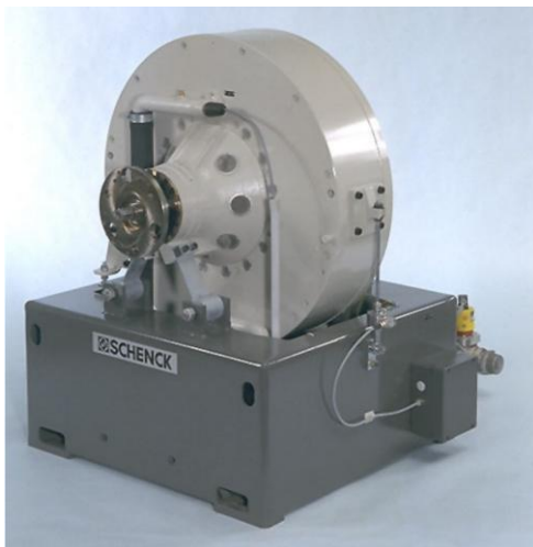
Figure 1 - Eddy current dynamometer (Schenck Pegasus, 2001)
