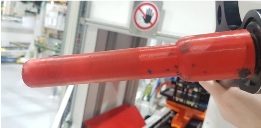
Figure 22: AM socket shroud after six months of use
