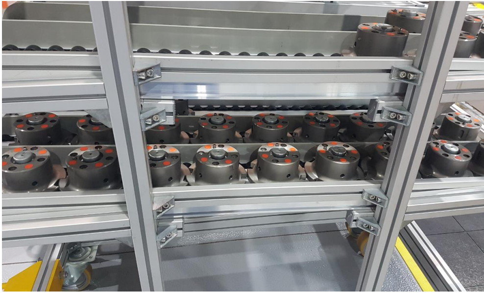
Figure 17: Cold test adaptors all with the AM seals fitted
