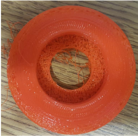
Figure 41: FDM seal with poor surface finish
