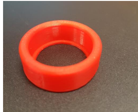
Figure 25: AM bearing cover created out of PLA
