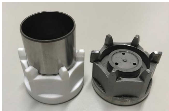
Figure 30: Tappet in 3D printed tappet gripper and non-AM tappet gripper
