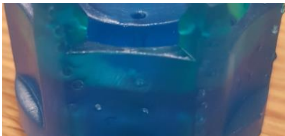
Figure 36: Scars on the SLA tappet gripper
