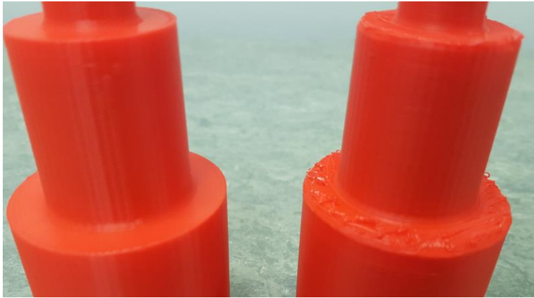
Figure 45: Left - component with good surface finish. Right - same component with surface scarring
