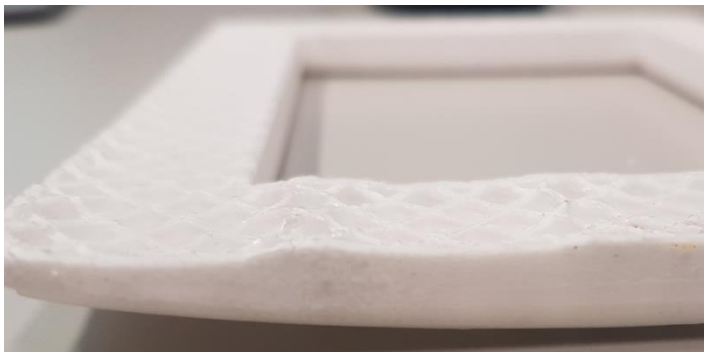
Figure 43: Component with poor bed adhesion
