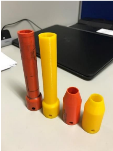
Figure 20: Socket shrouds, Orange are externally sourced, yellow are AM
