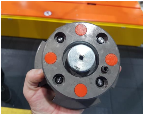
Figure 16: Cold test seals inserted into an adaptor
