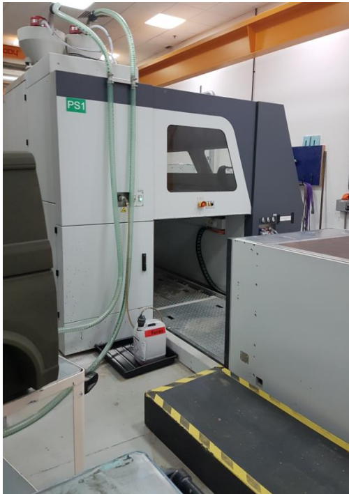
Figure 9: Dunton RP's sand printer
