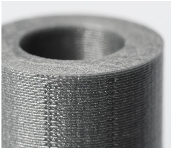
Figure 2: FDM product showing the layers that form during creation (Varotsis, 2019)
