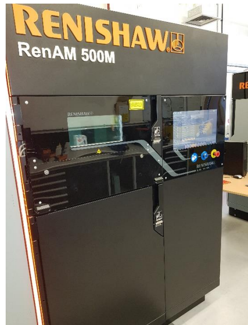
Figure 8: Renishaw SLM machine in Dunton RP
