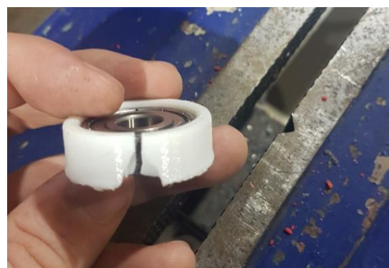
Figure 27: Split PC cover after bearing fitting
