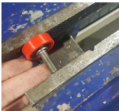
Figure 28: Bearing being fit into PLA AM cover
