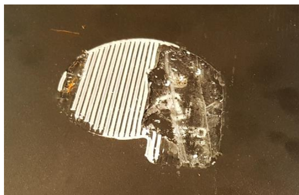
Figure 39: Damaged print bed
