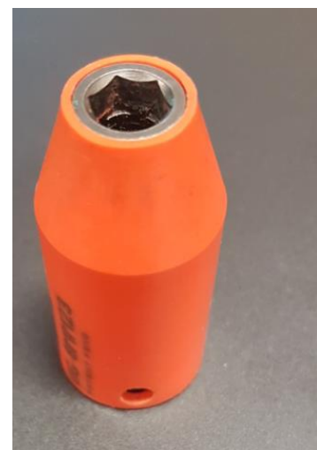
Figure 19: Socket with standard shroud fitted
