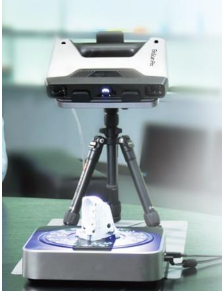
Figure 12: Einscan 3D scanner (Shining 3D, 2018)
