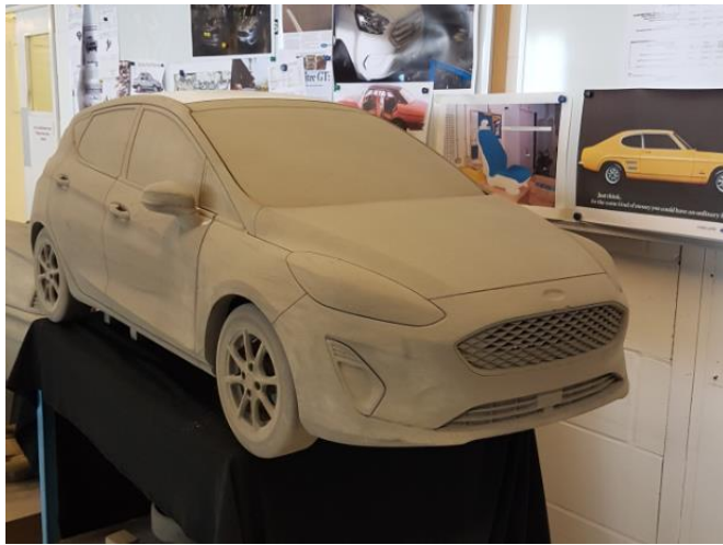
Figure 10: Model created by Dunton RP's sand printer
