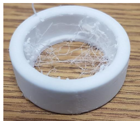
Figure 42: Igu bearing cover with stringing
