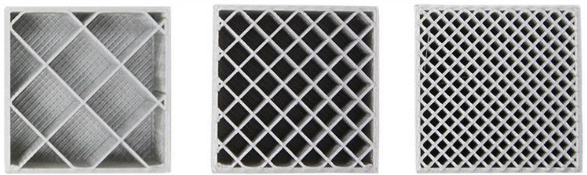
Figure 3: Different infill densities, 10% 25% and 50% respectively (Ultimaker, 2019)
