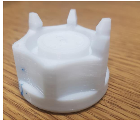
Figure 31: Damaged AM tappet gripper
