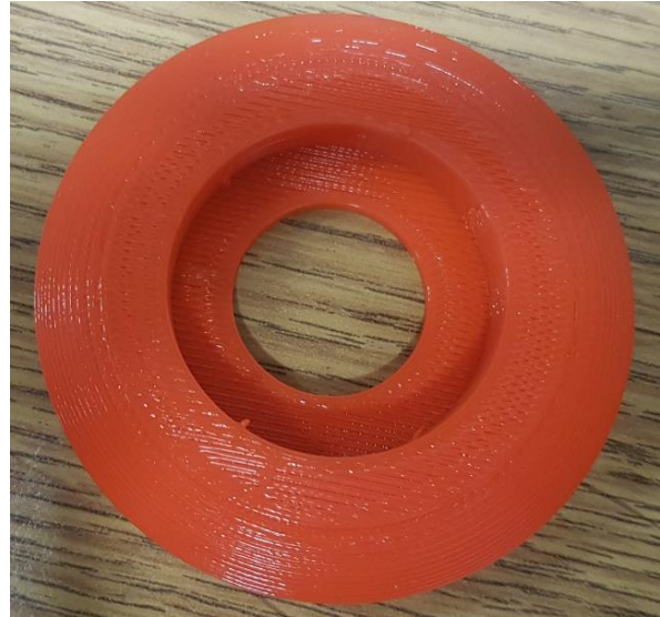
Figure 40: FDM seal with good surface finish
