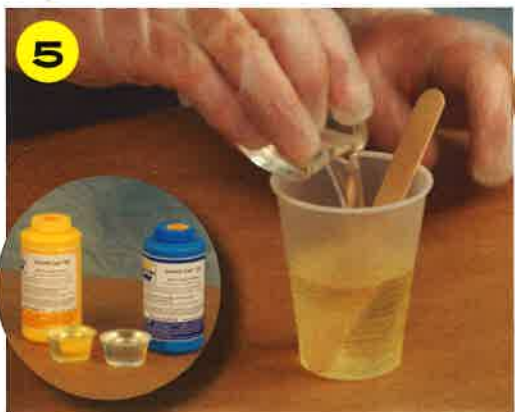
5 Smooth Cast® 300 is measured 1A:1B by volume. The two parts are combined.
