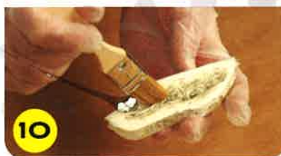
10 The mould is removed from the sculpt and cleaned with isopropyl alcohol and a brush.
