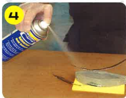
4 Universal Mold Release® is sprayed onto all surfaces.
