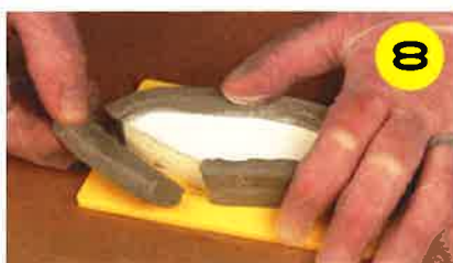
8 After the resin cures, the clay mould wall is removed.
