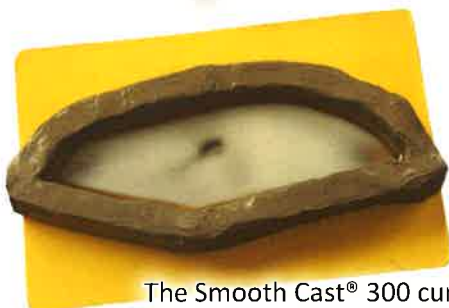
4 Universal Mold Release® is sprayed onto all surfaces.
