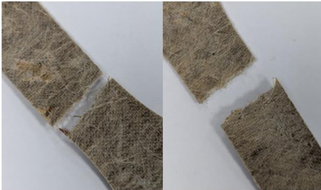
FIGURE 11: HEMP NON-WOVEN 3 x 100 BIO RESIN BREAK POINT
