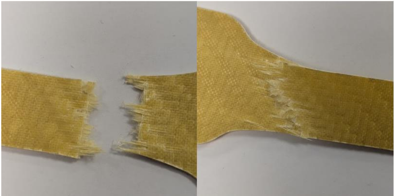
FIGURE 12: KEVLAR WOVEN 2 x 300 BIO RESIN BREAK POINT
