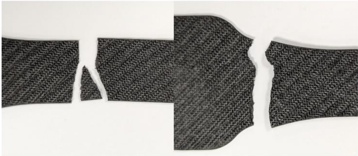
FIGURE 8: CARBON FIBRE NON-WOVEN 1 x 300 BIO RESIN BREAK POINT
