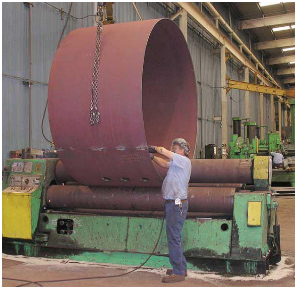
Figure 4. Formed shell strake (Hurst Boiler, 2018)
