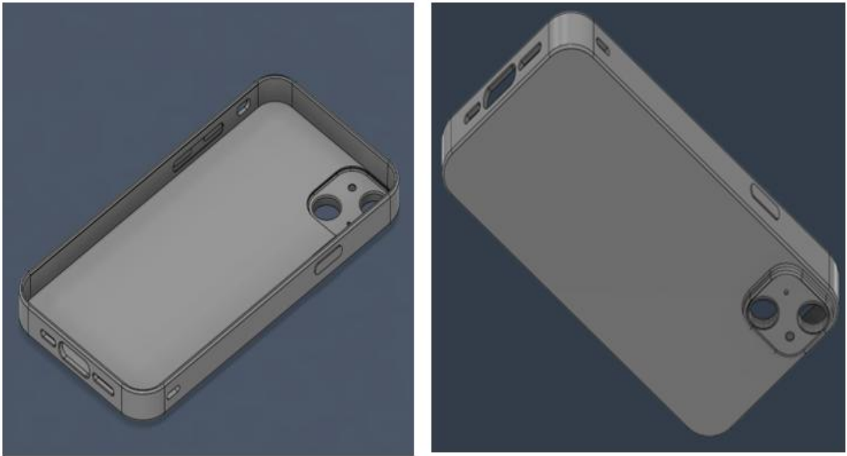
Figure 3: Final CAD model of the mobile phone housing developed in Autodesk Fusion 360.
