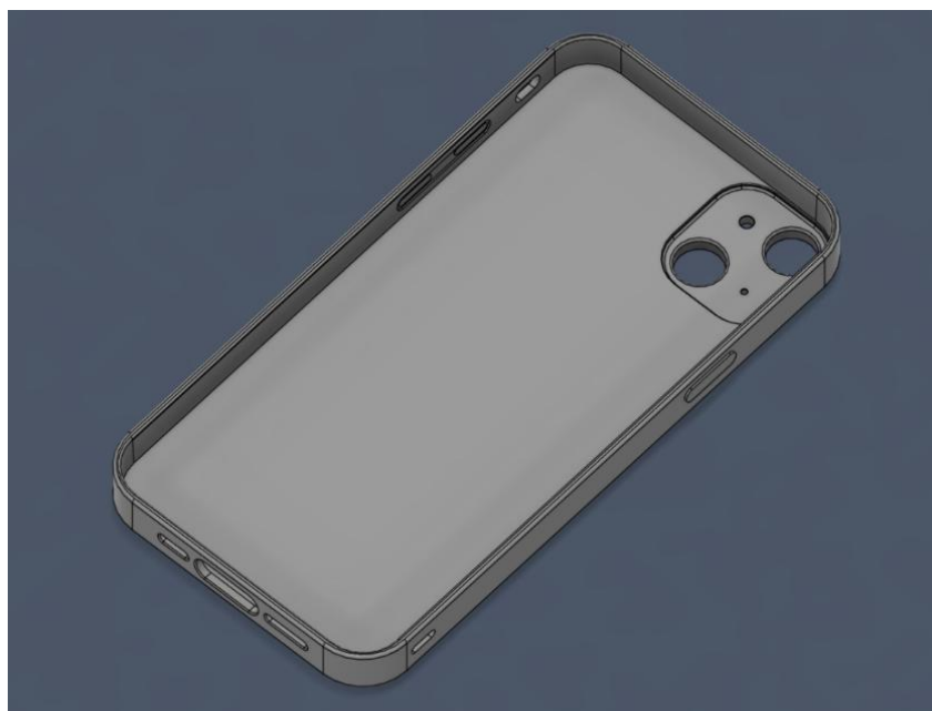
Figure 2: Baseline design of the mobile phone housing in Autodesk Fusion 360
