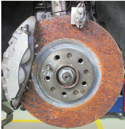
Figure 23 Corroded Brake Disc (The Brake Report, 2020)
