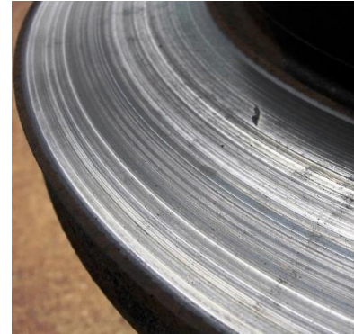
Figure 11 Worn Brake Disc (The Filter, 2018)
