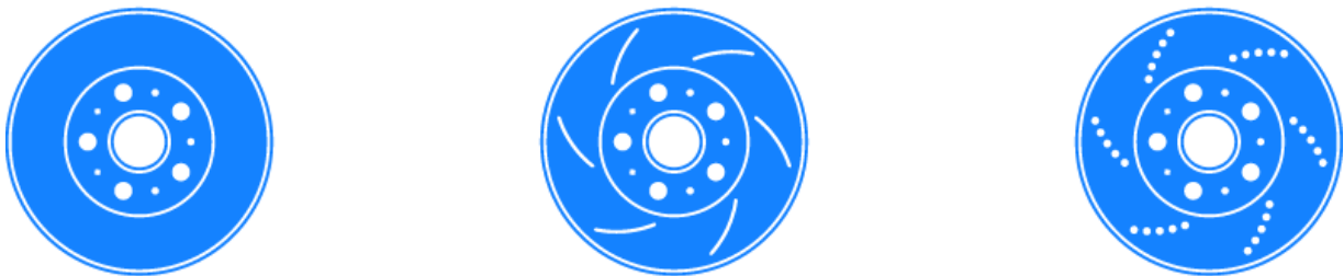
Figure 3 Smooth, Slotted and Drilled Brake Discs (NewParts, 2020)
