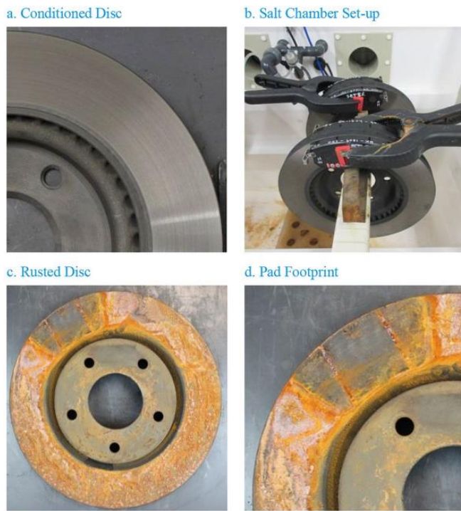
Figure 21 Disc-Brake Corrosion Procedure (Ferrer, 2019)
