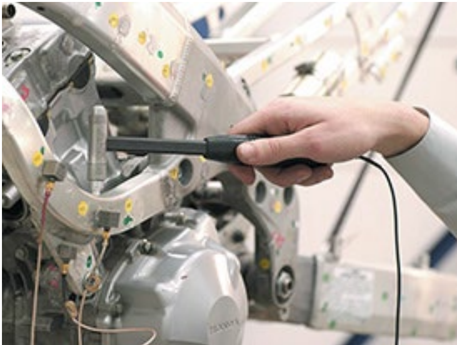
Figure 11 Hammer test of motorcycle chassis with engine (Siemens, 2019)
