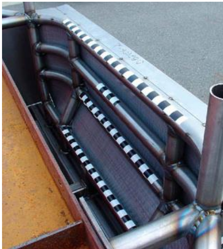
Figure 2.1: Tegrise composite shown in the crash structure of a NASCAR (Hayes, 2008)
