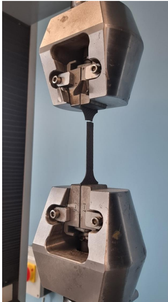
Figure 3.1: Denison tensile test rig post sample test
