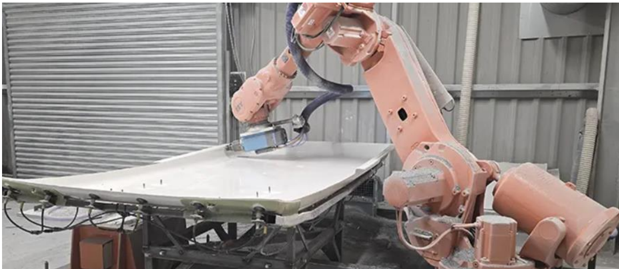
Figure 5.3: Composite trimming robot increasing fabrication energy requirements (Quantum Mouldings Ltd., 2026)
