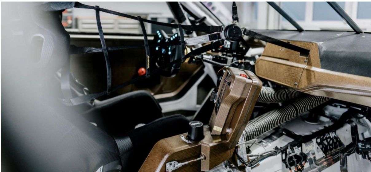
Figure 2.6: The interior of the BMW M4 GT4 racing car with Bcomp natural fibres visible on the centre console (BMW M, 2022)
