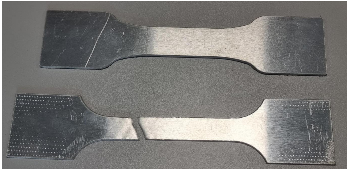
Figure 4.9: Aluminium sample before (top) and after tensile test (bottom)
