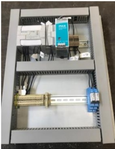
FIGURE 40 - PLC MOUNTING PANEL
