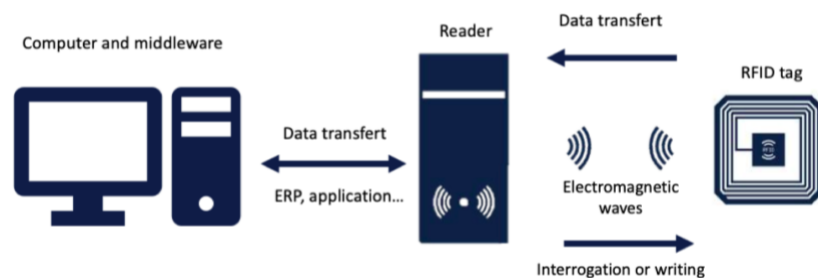
Figure 2: Operating diagram of RFID technology
