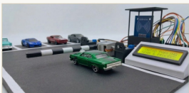
FIGURE 3 – ASSEMBLED PROTOTYPE WITH IP65 ENCLOSURE, NFC READER, AND SOLAR PANEL.
