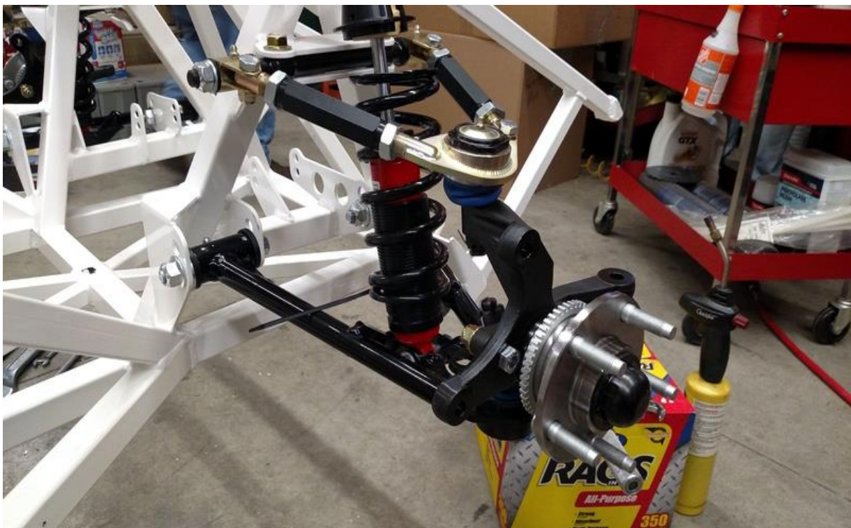
Figure 2 – Double Wishbone Suspension (image courtesy of FactoryFiveRacing)
