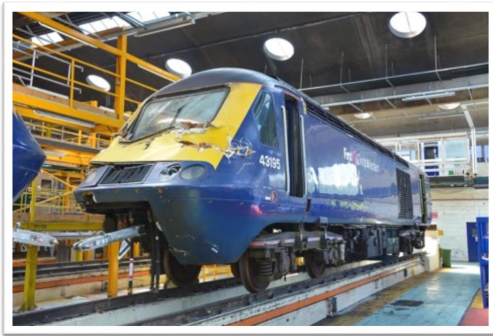
Figure 3: Power car no. 43195 has sustained unforeseen damage. It is currently being used as a spares donor
