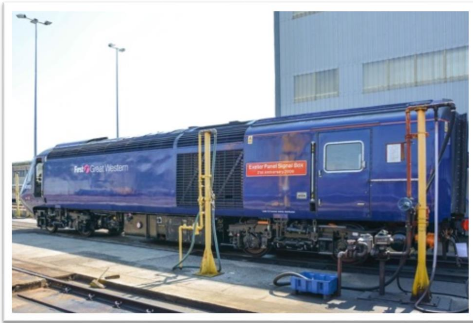
Figure 2: Power car no. 43162 has received new wheels as part of a 'G' exam
