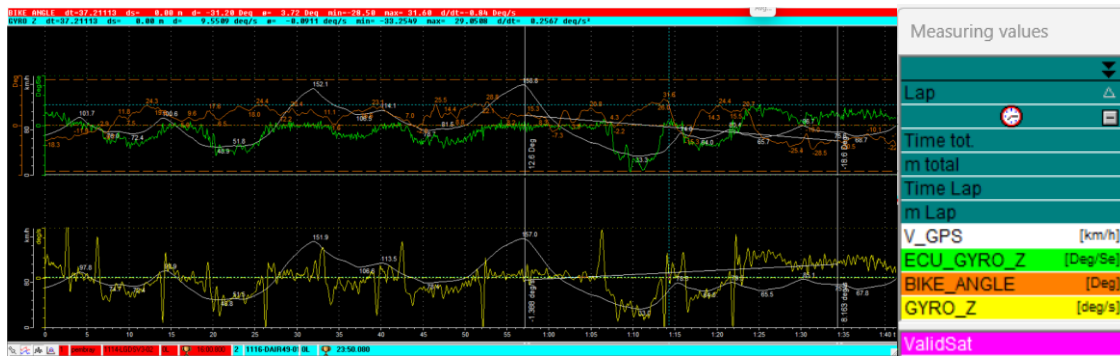
Figure 10: Pembray rider lateral roll rate (lower trace) compared with bike lateral roll rate (upper trace)
