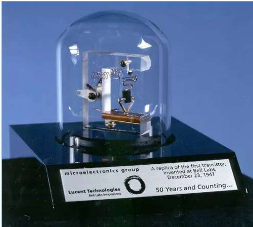
Figure 2: Replica of the world's first semiconductor transistor, invented at bell labs by physicists William Shockley, Walter Brattain and John Bardeen 1947.[3]
