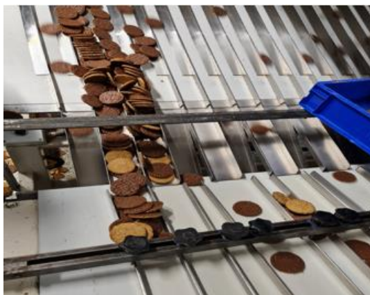
Figure 20- Biscuits stuck in-between guide.
