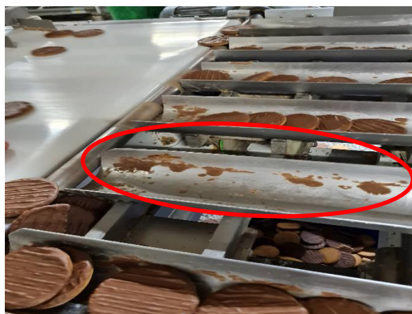
Figure 22- Excessive chocolate build up from inadequate cooling.
