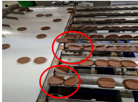
Figure 25- Trapped biscuits from not having a guide.
