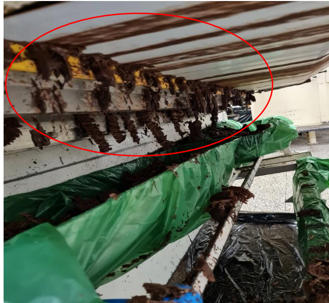
Figure 16- Build-up of chocolate on enrober scraper.
