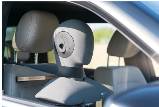
Figure 1 – An artificial head with microphones to record the sounds an occupant hears (Continental Engineering Services, no date).
