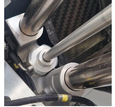
[Figures 2.2.1 & 2.2.2] Hydraulic control system of the rear wing. (photos by Catriona Burn)
