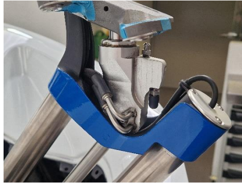
[Figures 2.2.1 & 2.2.2] Hydraulic control system of the rear wing. (photos by Catriona Burn)
