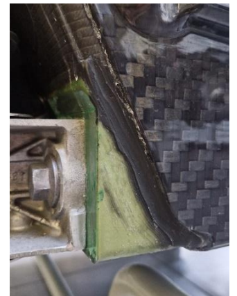
[Figure 2.1.3] Aluminium bonded to carbon fibre with a strong resin. (photo by Catriona Burn)
