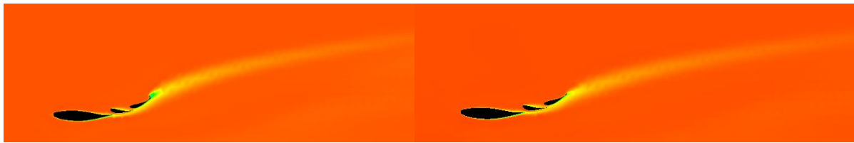
Figure 94 - Total Pressure Contours (Left - Gurney Flap, Right - No Gurney Flap)
