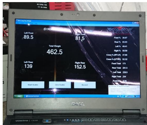
Figure 6 - SBD Ltd Dallara F399/01 Corner Weights (Kg)
