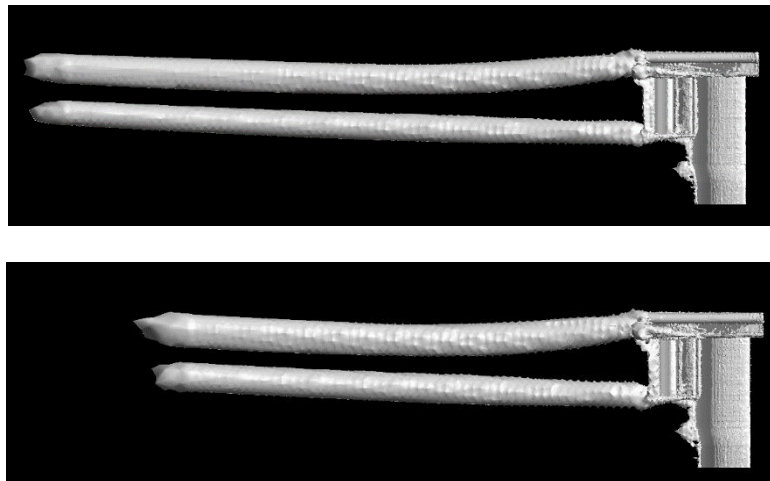
Figure 97 - Vortex Swirling Strength (Top - No Gurney Flap, Bottom - Gurney Flap) (0.01Hz)
