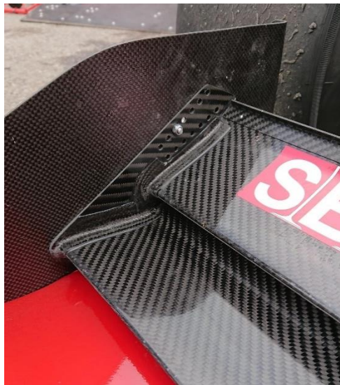
Figure 48 - F399 Front Wing Flap Adjustment
