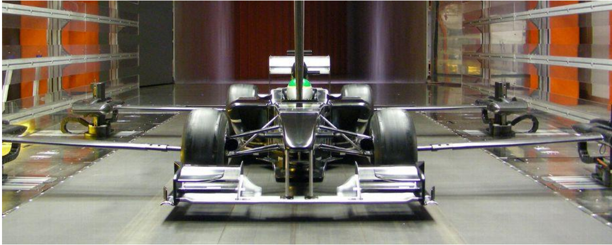
Figure 18 - Wheels Off Wind Tunnel Test (Edmondson, 2015)
