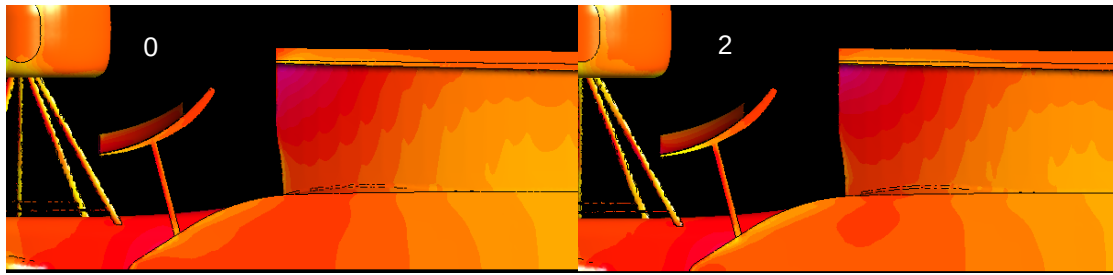
Figure 144 - Floor Static Pressure Contours
