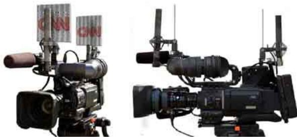
Fig. 14: Two BPT-Mics mounted ‘back-to-back’ on video-camera , with acoustic panels
