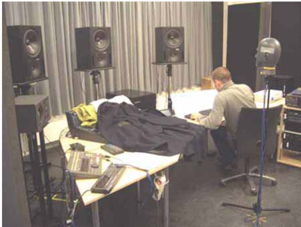
Fig. 10: Re-recording of the surround-microphone signals at sweet spot of the control room at the IEM (rear channel loudspeakers outside of the picture)
