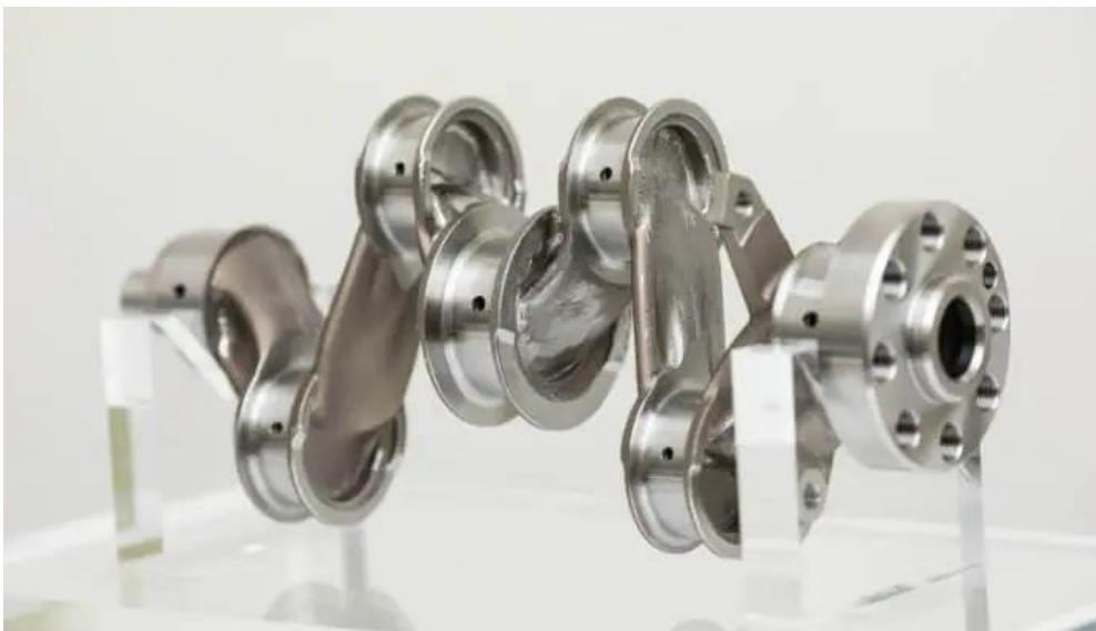
Figure 7. The metal-printed prototype for the generative-design crankshaft model. (Matsunaka, 2022)
