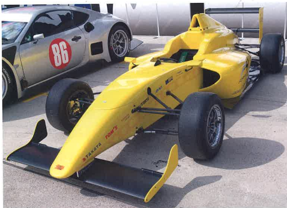
Dome F110 in standard F4 trim. ERA has designed a frame for the rear so the suspension pick-ups will remain the same
