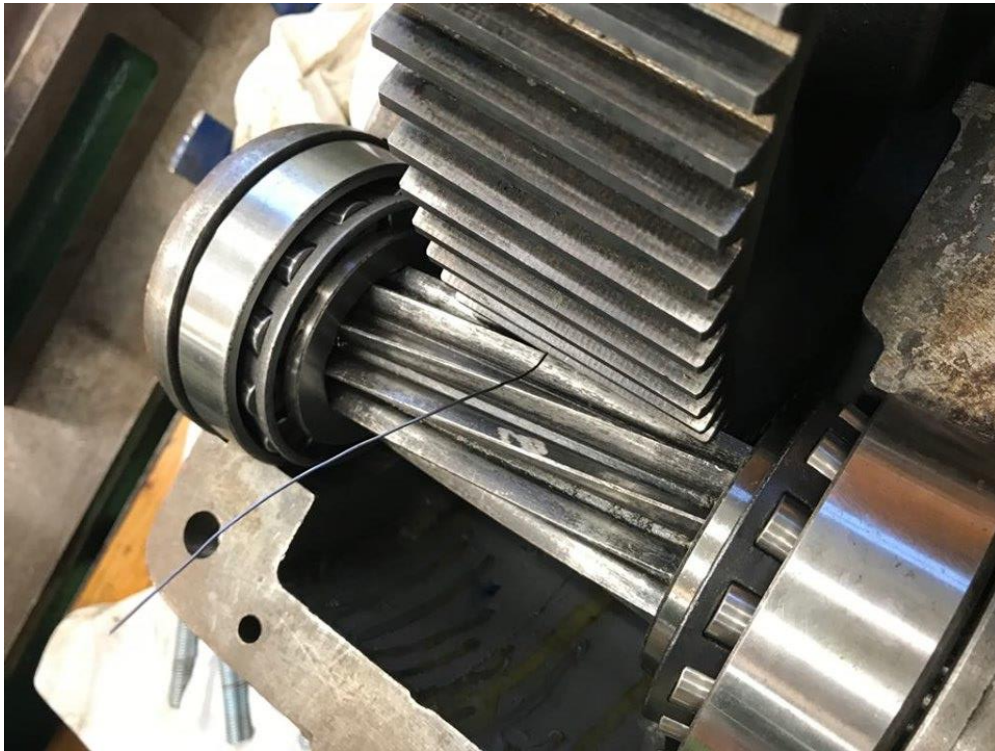
Figure 16 Measuring clearance between the gear's teeth
