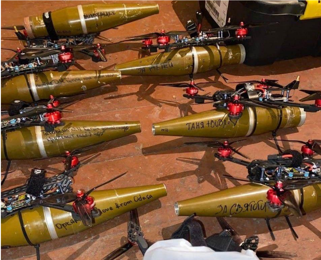
FIGURE 12 - UKRAINIAN FPV DRONES CARRYING MUNITIONS UP TO 2KG [23]
