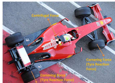
Figure 2 shows how forces are exerted on the tyres while cornering and the centrifugal forces exerted on the centre of mass.
