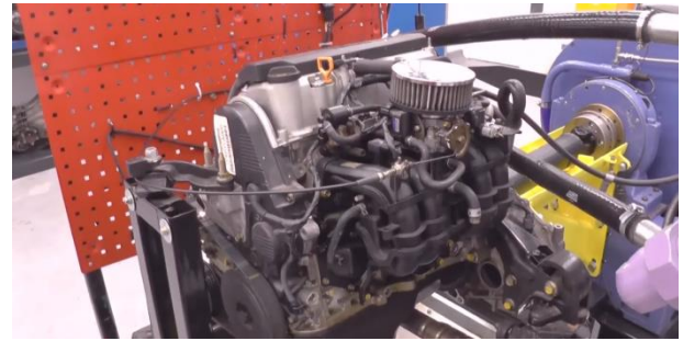
Figure 2: Engine, mounted to Dynamometer
