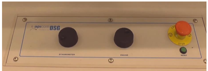
Figure 4: Dynamometer controls from within Dyno cell
